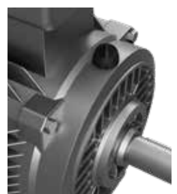
Vibration - magnet mounting
